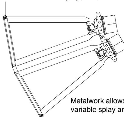
Metalwork allows for variable splay angle
